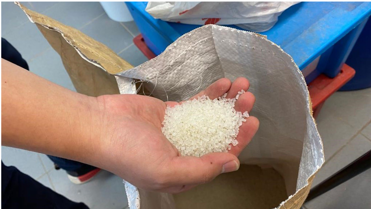
With each particle measuring 2mm to 4mm, the plastic waste (polypropylene) aggregate is now ready for use in the concrete mix.
