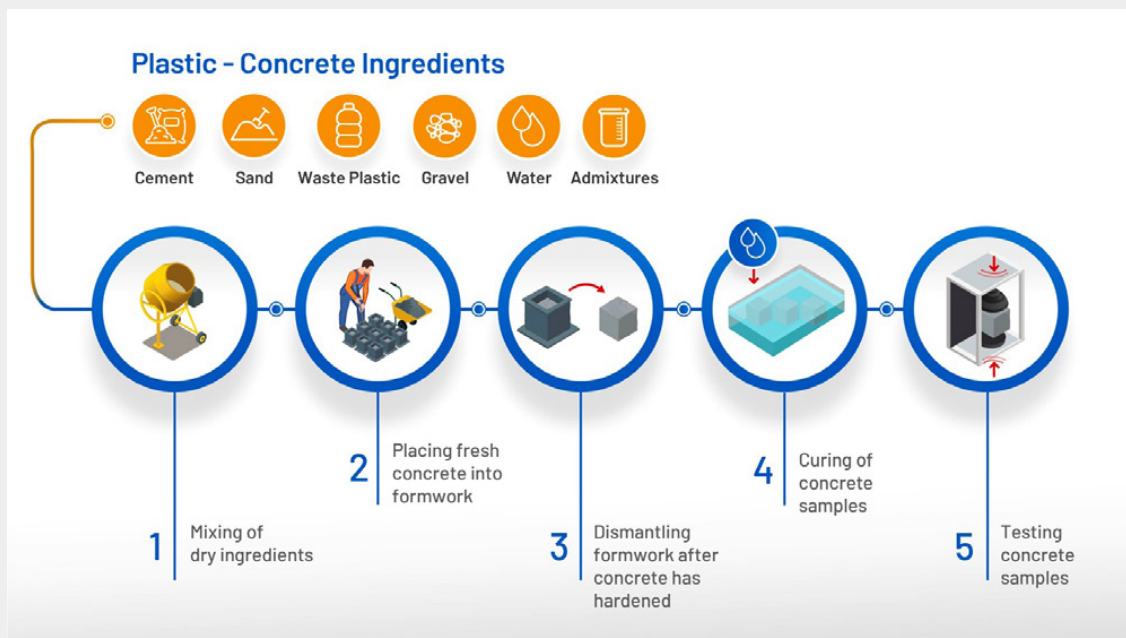
The process of mixing the plastic-concrete mix, and then forming, curing and testing the performances of the samples.
