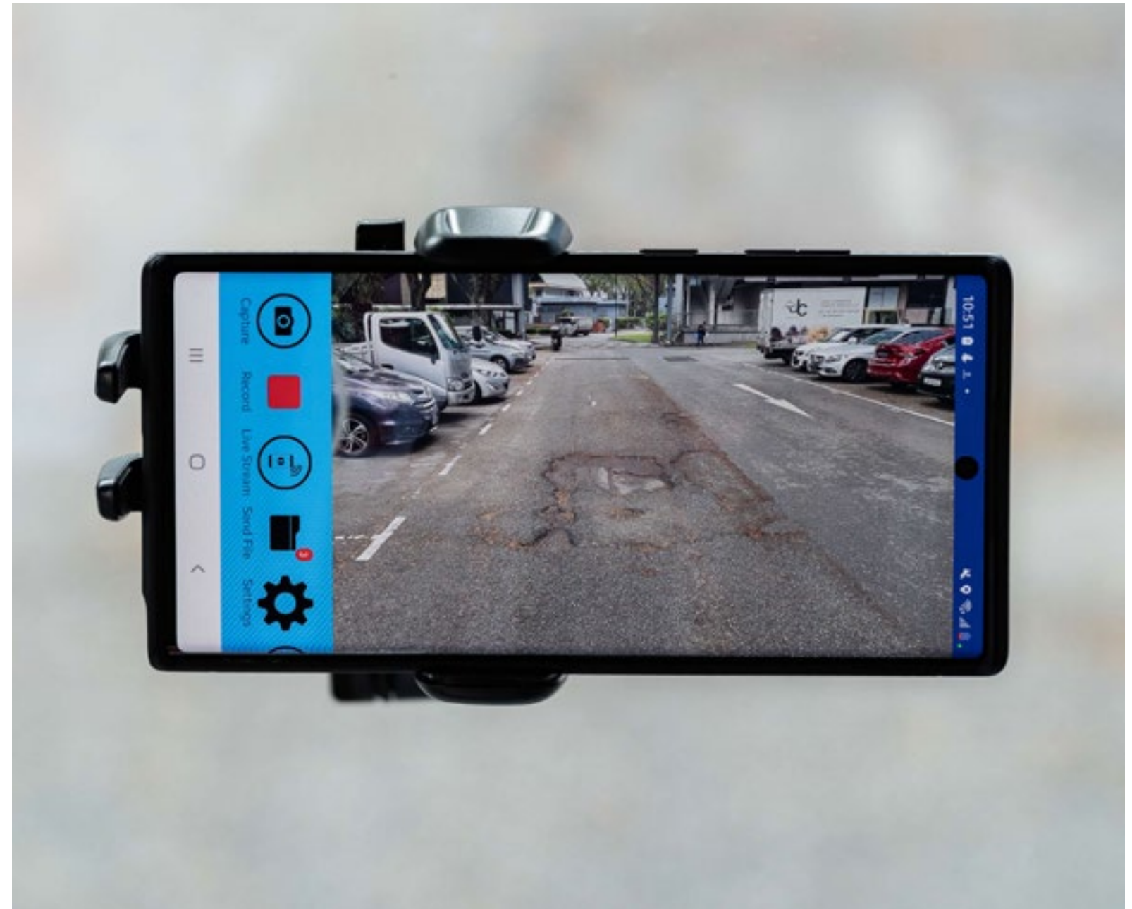
The brainchild of JTC and Vebits AI, our new solution for estate inspections blends the use of smartphones, AI, and real-time machine vision. Since November 2022, it has been deployed at one-north.
