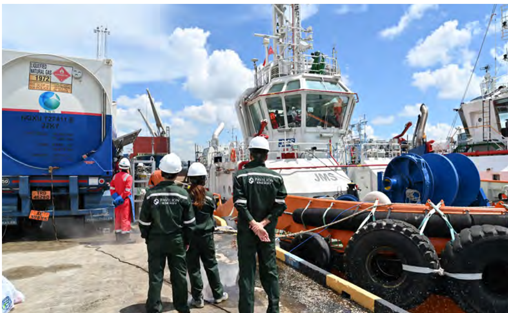
Bottom: LNG truck-to-ship bunkering operation for JMS Sunshine (Credit: Pavilion Energy)
