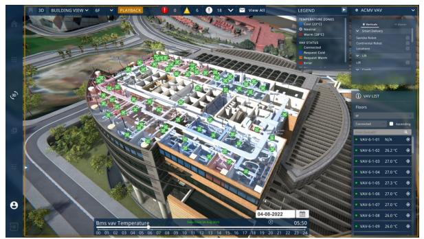
Historical data can be saved and played back to aid troubleshooting for facility management-related issues. This includes identifying cooling system issues such as aircon failures or airflow restrictions.
